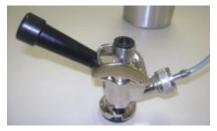
STEP 6 After the backflow stopper has been inserted, there is a washer that should be placed on top of the coupler.
